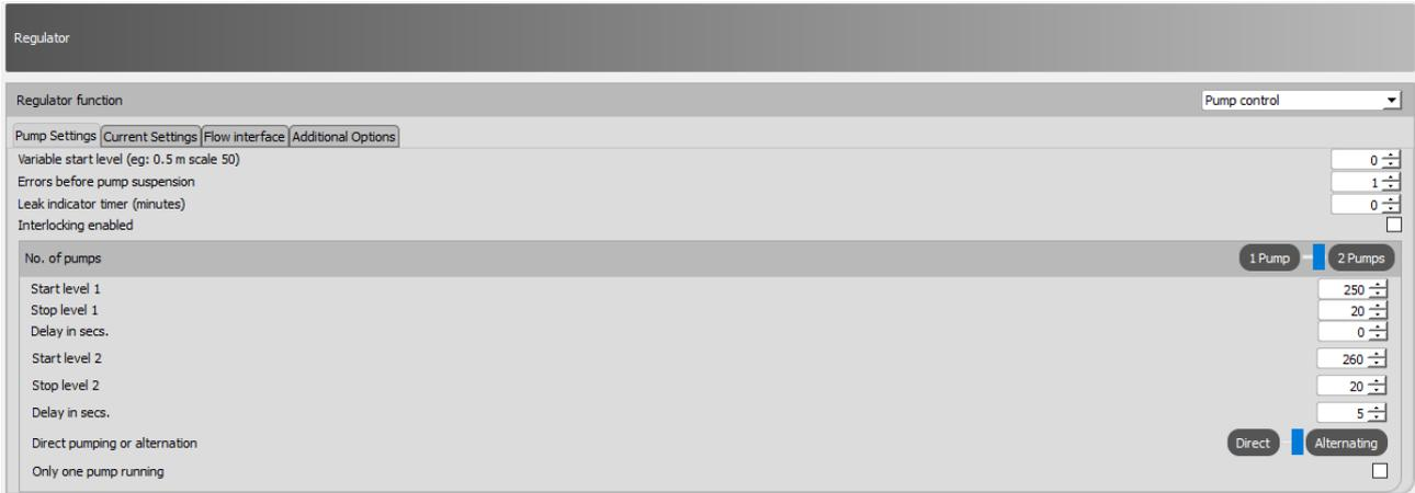
In order to use SPIDER as a pump control, select "Pump control" under the "Regulator function" setting. Here you can configure the most common parameters as shown in the picture.
