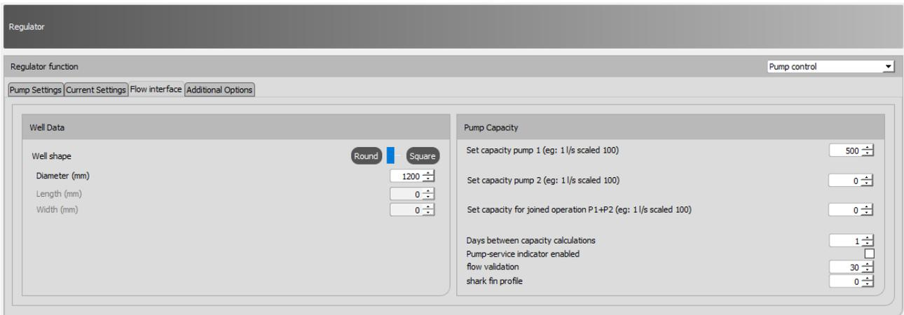
With very few settings, SPIDER can perform a validated flow calculation. You choose whether the shape of the well is round or square, then enter either diameter or the dimension of the sides in mm. This determines the surface area and SPIDER calculates based on the start/stop levels how much is pumped out during a pumping cycle.
