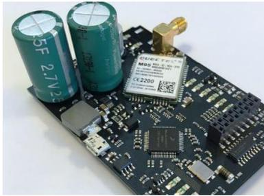
SPIDER is equipped with a built-in Power bank and can send voltage failure alarms when the primary power supply disappears.
